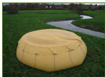
It is necessary to adjust the tension on the ropes as the water level of the tank fluctuates, during the filling/emptying operation.
