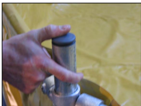
11. Fit 2" nipple and ball valve. (*not supplied*)
