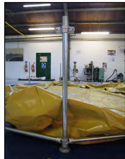
6. The horizontal pole, where the outlet is positioned, can be raised to accommodate the outlet, if required.
