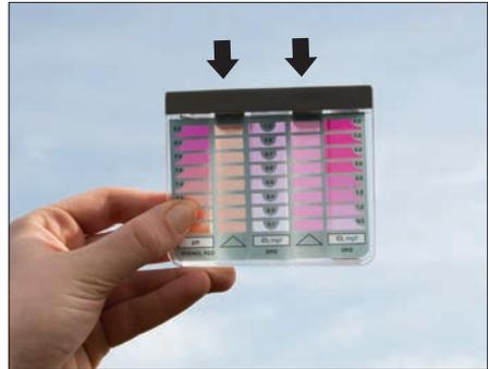
**4** Immediately read the free chlorine residual (mg/litre) and pH by holding the comparator up to daylight and matching the colour in the cells with the standard colour scales. If the colour falls between two standard colours, then it will be necessary to estimate the concentration.
