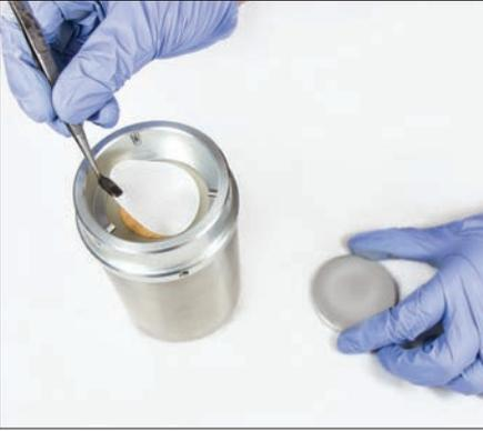
**14** Unscrew the collar and remove the funnel and collar with one hand. Using the sterilised tweezers in the other hand, lift the membrane carefully from the filtration base. Hold the membrane by the edge only.
