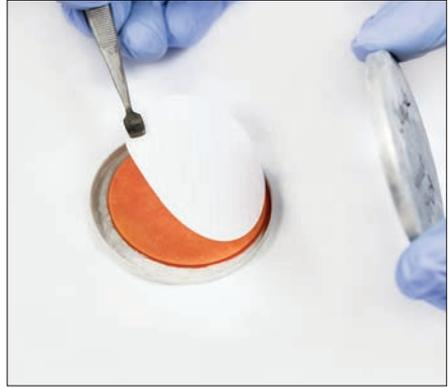
**15** Remove the lid of a prepared petri dish and place the membrane, grid side up, onto the absorbent pad soaked in culture medium. Start at one edge (it is easier to use the one at a greater distance from the wall of the petri dish) and lower the membrane on to the pad by 'rolling' so as to avoid trapping air bubbles under the membrane.
