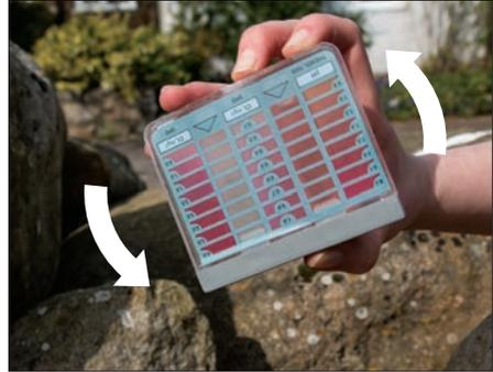
**6** Again, invert the comparator several times to dissolve the tablet. Leave the colour to develop for **10 minutes**. Read the total chlorine residual (mg/litre) by matching the colour in the cells with the standard colour scale (as shown in the image below).
