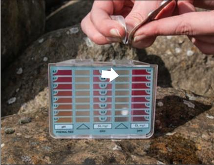
**5** To test for total chlorine residual, **DO NOT** discard the liquid in the comparator. Remove the lid and add one DPD No.3 tablet to the right hand cell (Cl<sub>2</sub>).
