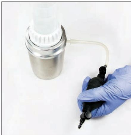
When all the water has passed through the filter, disconnect the pump from the filtration apparatus. **DO NOT** allow excess air to be drawn down through the filter once all the water has gone through. ►
