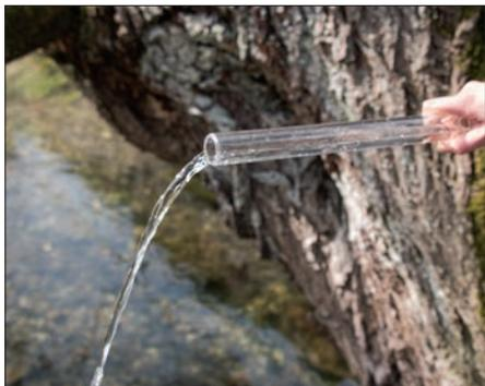
**4** Alternatively, the procedure can be carried out in reverse by filling the tube with the sample and then slowly pouring out the water. Keep pouring until the black marker is visible.
