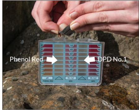
**2** Drop one DPD No.1 tablet into the right hand cell ( $\text{Cl}_2$ ) and one Phenol Red tablet into the left hand cell (pH).
