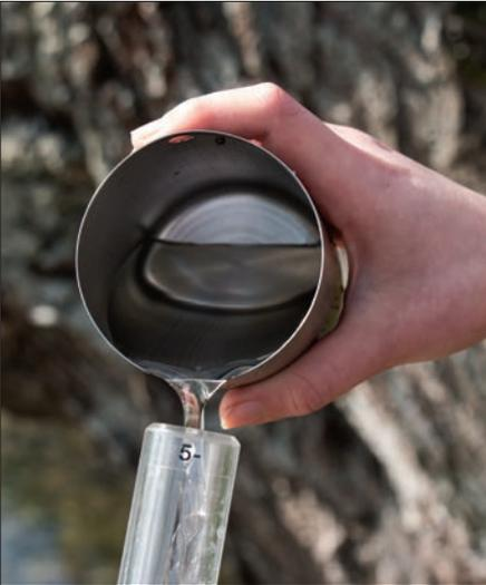
**3** Hold the tube vertically and slowly pour the water sample into the tube until the marker disappears when viewed from the top of the tube. Avoid creating bubbles, as this may cause false readings.
