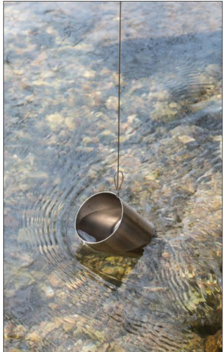
**i Note:** It is important that you obtain a sample which is representative of the main body of water. For example, when sampling from a river, **DO NOT** sample the quiet or stagnant areas near the bank, as these do not represent the main body of water. Furthermore, it is vital not to introduce external contamination into the sample. For this reason it is often better to sample with the help of the cable supplied with the kit.
