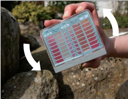
**3** Replace the lid of the comparator and push down firmly to seal. Invert the comparator several times until the 2 tablets have dissolved completely. If the tablets are slow to dissolve use the plastic paddle from inside the box of tablets to crush and mix the tablets in the sample water.
