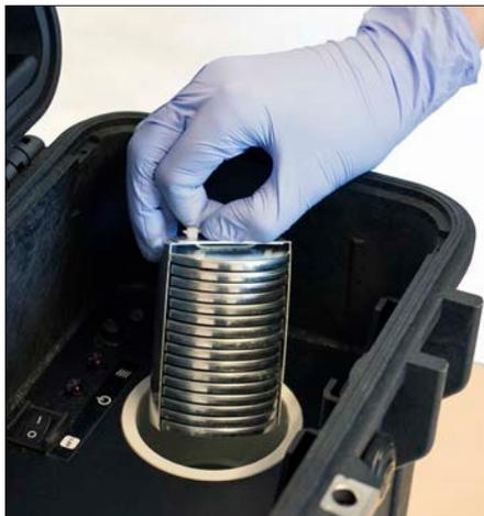
**18** Resterilise the filtration apparatus (Section 3.1). ◀
