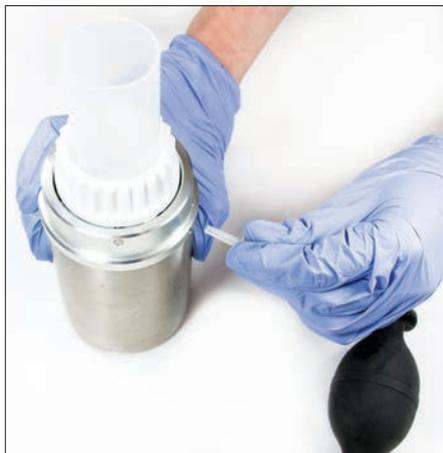
**13** Insert the plastic connector of the vacuum pump into the vacuum connection on the filtration base. Squeeze the pump bulb several times to draw a vacuum, then squeeze as required to draw all the water through the membrane filter.
