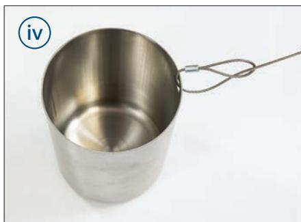
**1** To fasten the sampling cable to the cup, feed the looped end of the cable through the hole in the side of the cup. Pass the other end of the cable through the loop and pull firmly. *Alternatively*, the clip on the end of the cable can be fastened to the hole.
