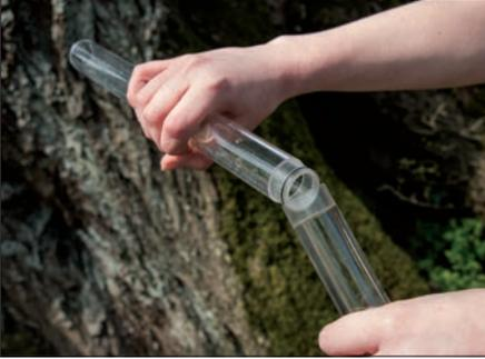
**1** Carefully remove the 2 halves of the turbidity tube from their clips in the lid of the case. Push the upper tube (open at both ends) squarely into the lower tube and align the graduation marks up the side.
