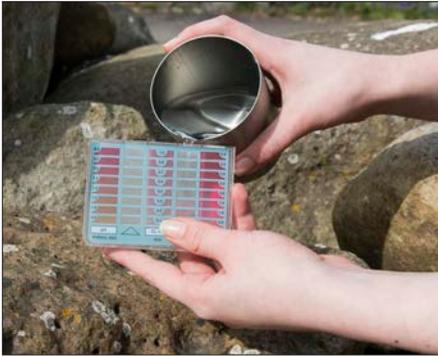
**1** Wash the comparator cells **three times** with the water that is to be analysed and then fill both cells with the sample.
