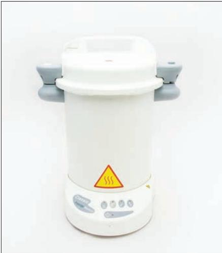
**5** If an autoclave is available (above), sterilise the bottles at **121°C** (equivalent to 1 bar, or 15psi steam pressure) for **15 minutes**. Tighten the caps carefully once the medium has cooled.
