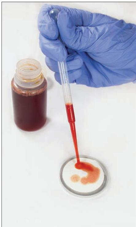
**1** Using the absorbent pad dispenser, place one pad into each petri dish (this operation may be done at base before leaving for the field).
