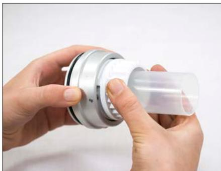
**1** Take the plastic collar and secure the filtration funnel in the loose but not free position (see [Section 5.4.3 \[pg. 35\]](#)) which will allow the formaldehyde gas to penetrate all areas of the filter head. ▶
