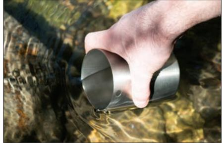
**2** Submerge the cup about 30cm below the surface of the water and scoop up the water sample (as shown in the top right image). This scooping action ensures that no external contamination enters the sample cup.
