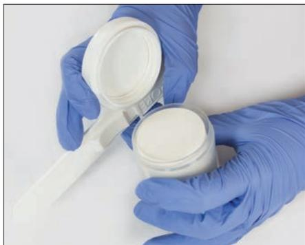
The pads are supplied sterile in packs of 100 units. A pad dispenser is also supplied with the kit. **NEVER** leave the dispenser without a pack of pads attached as it will increase the possibility of contamination. If the dispenser is lost or damaged, pads may be dispensed in the field using the sterile tweezers (see [Section 5.4.3 \[4\]](#) for sterilisation methods). ▶
