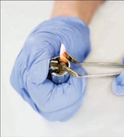
**4** To sterilise the tweezers, flame the tips with a lighter for approximately 5 seconds and leave to cool.
