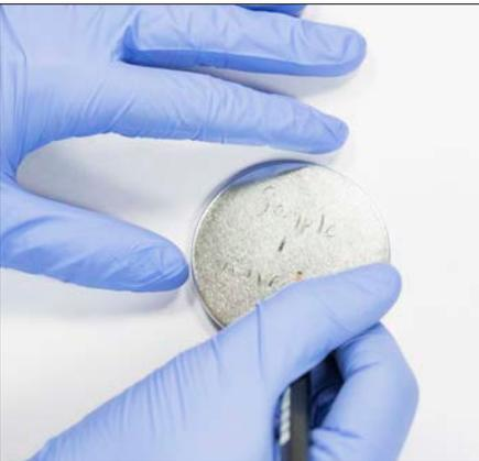
**16** Replace the lid of the petri dish and mark the lid with sample information e.g. volume filtered, source, time and date; or a code which relates to details on the daily report sheet. A wax pencil or marker pen is suitable for this purpose (the writing needs to be easily removed after the tests are complete). ▶
