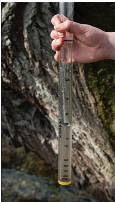
**5** Hold the tube vertically and read the turbidity using the graduations on the side of the tube (as shown in the image to the left). The result is the value of the line nearest the water level.
