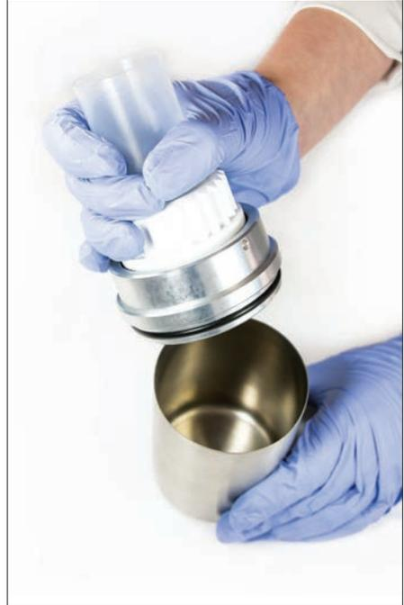
**5** Push the filtration apparatus firmly onto the vacuum cup. If this is difficult, lubricate the black rubber O-ring with silicone grease.
