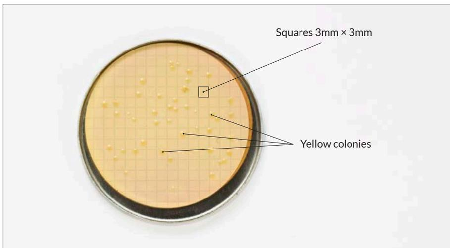
**1** Once the incubation period is complete, remove the petri dishes and their holder from the incubator. Carefully lay the plates out, in sample order, on a table to allow effective results comparison.
