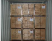
The T12SLR O2 tank (11,983 litre capacity) is designed to fit within the racks of most racking systems in use around the world. You asked us for this feature & we delivered. The new packing cases also include pre-positioned carry stretchers that enable the tank components to be transported over broken ground using manpower alone : reliance on mechanical handling is no longer necessary.
