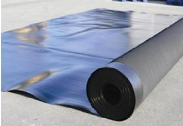
A high quality, single layer HDPE suitable for use as a barrier membrane on brownfield sites, petrol stations, coalfields, landfill & contaminated industrial areas. The material is highly suited to attenuation ponds, lagoons, water features & as a high performance damp proof membrane because of its high puncture resistance. The membrane offers protection from Carbon Dioxide, Methane and Radon as well as certain common hydrocarbons.
